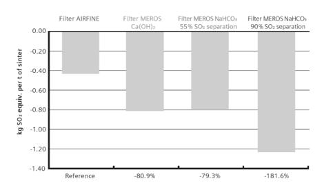
• Gas cleaning with the Airfine process was used as a reference
