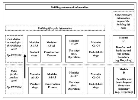
Fig.1: Schematic modular structure of building and product life cycle stages according to CEN TC 350.
