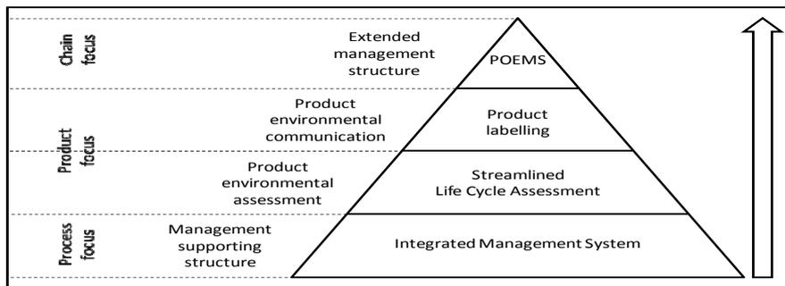
**Fig.1: The modular structure of the POEMS framework**
